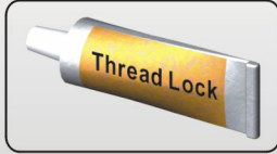
Threadlock Threadlock should be used wherever a metal screw is being fastened into a metal part. Threadlock prevents the screw from loosening due to vibration.
