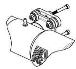
Note: Between the engine exhaust port and the manifold surfaces, add a thin layer of 5 minutes epoxy glue to ensure a gas seal. Re-check all 6 screws after the first few flights with a warm engine.
