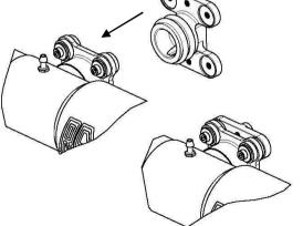
STEP 4: Insert the manifold into the muffler and lock the screws with loctite (medium strenght )
